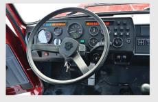
System reliability increased and the steering wheel can now be easily rotated. Modern motor is controlled by an electronic accelerator, in the new dashboard is an electronic speedometer and tachometer.
